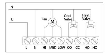
**Note:** CO--Cool Valve Open CC--Cool Valve Close HO--Heat Valve Open HC--Heat Valve Close
